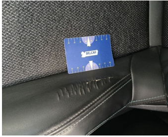
Seat Front Left / Bottom Coating / Replace-worn
