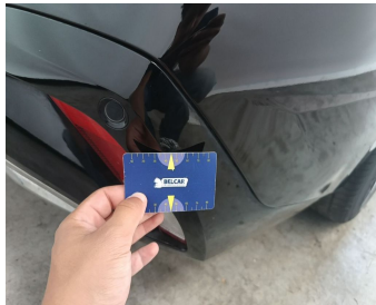
Bumper Rear // Smart Repair Medium-scratch
