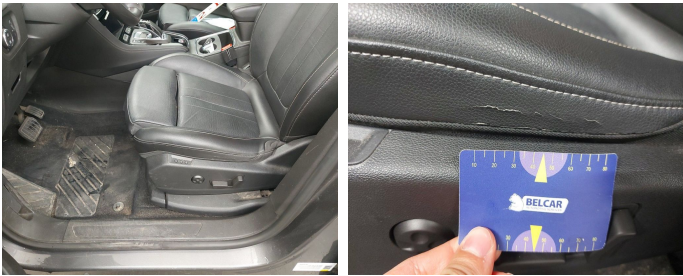
Seat Front Left / Bottom Coating / Replace-worn
