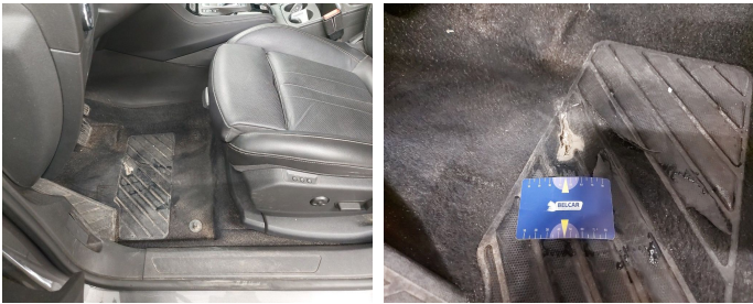
Interior / Floor Covering / Replace-worn
