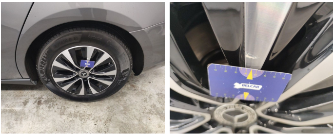
Wheel Two Tone Rear Left // Repair-scratch
