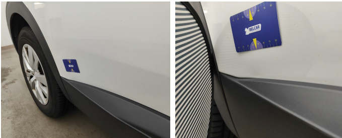
Door Rear Right // Smart Repair Small-dent
