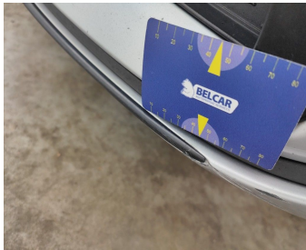
Bumper Front / Trim Left / Replace-scratch
