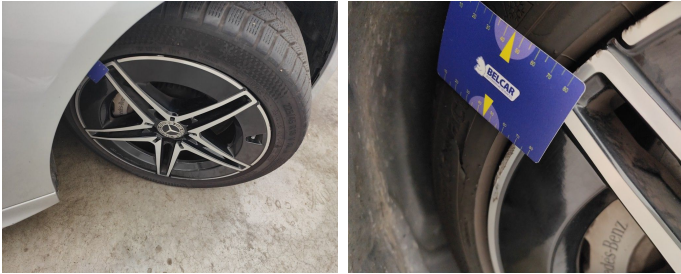
Tyre Front Right // Replace-tear
