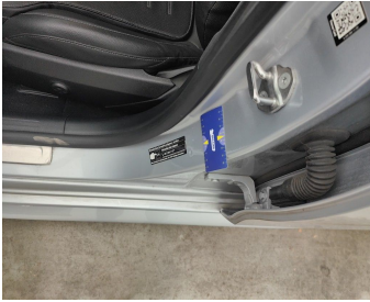
Rocker Panel Left // Smart Repair Medium-scratch + dent
