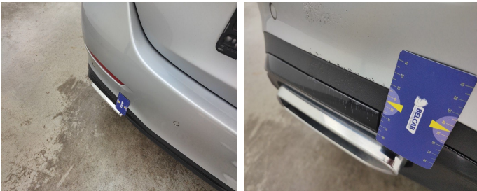
Bumper Rear / Spoiler / Replace-scratch
