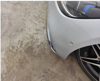
Bumper Front / Trim Left / Replace-scratch
