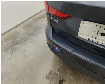
Back Side / Reflector L / Replace-scratch
