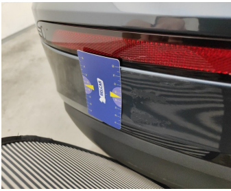
Bumper Rear // Repair & Painting-cracked
