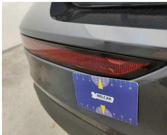
Back Side / Reflector L / Replace-scratch
