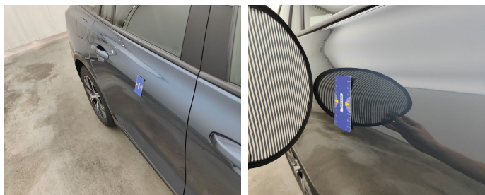
Door Rear Right // Repair & Painting-scratch + dent
