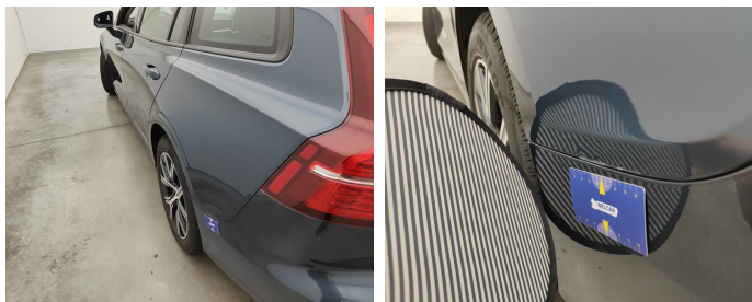
Wing Rear Left // Repair & Painting-scratch + dent
