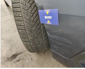
Bumper Front // Repair & Painting-scratch
