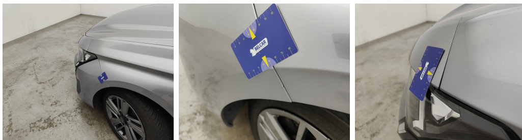
Bumper Front // Repair & Painting-bad repair
