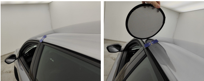
Roof // Smart Repair Medium-dent
