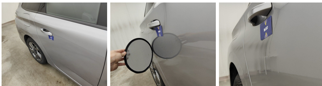
Door Rear Right // Painting-bad repair
