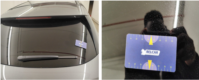
Rear Bonnet / Rear Window / Replace-scratch
