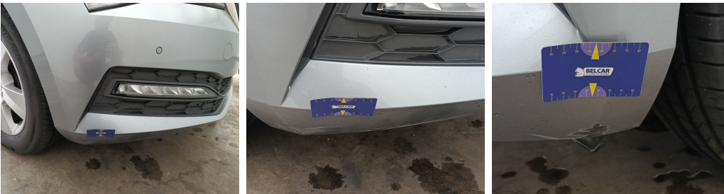
Bumper Front // Smart Repair Large-scratch
