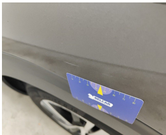
Bumper Rear // Repair & Painting-scratch
