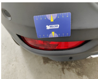
Back Side / Reflector R / Replace-bad position
