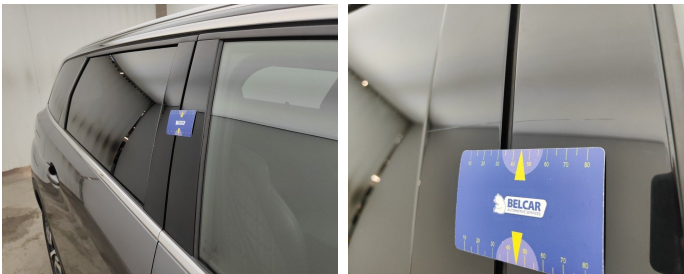
Door Front Right / Trim / Replace-scratch
