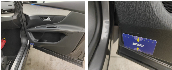
Front Right Door Interior Coating // Replace Completely-scratch
