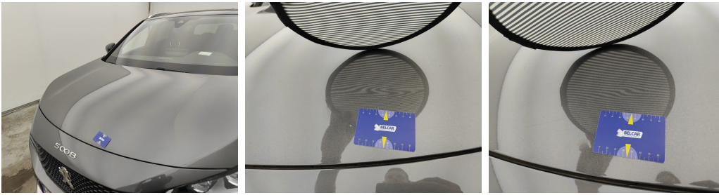
Front Bonnet // Smart Repair Small-dent
