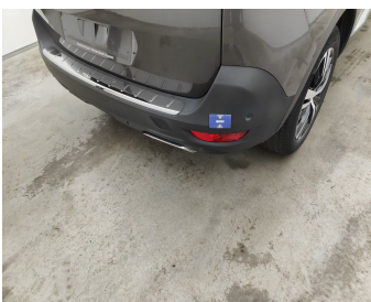
Back Side / Reflector R / Replace-bad position
