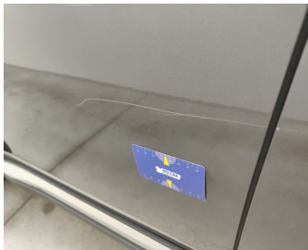
Door Rear Left // Repair & Painting-scratch + dent
