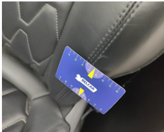
Seat Front Left / Rear Coating / Replace-worn
