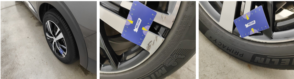
Wheel Two Tone Rear Left // Repair-scratch
