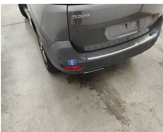
Back Side / Reflector R / Replace-bad position
