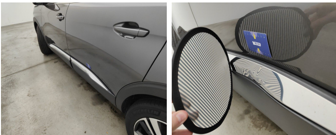
Door Rear Left / Trim / Replace-dent
