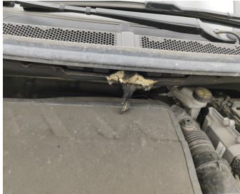
Engine Compartment / Silencer / Replace-tear
