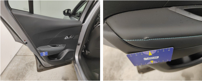
Rear Left Door Interior Coating // Replace Completely-scratch
