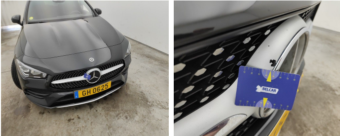
Front / Logo / Replace-Chipped paint
