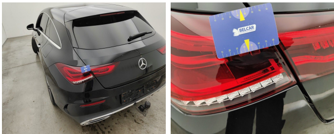
Light / Rear left / Replace-scratch
