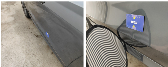
Door Front Right // Repair & Painting-scratch + dent
