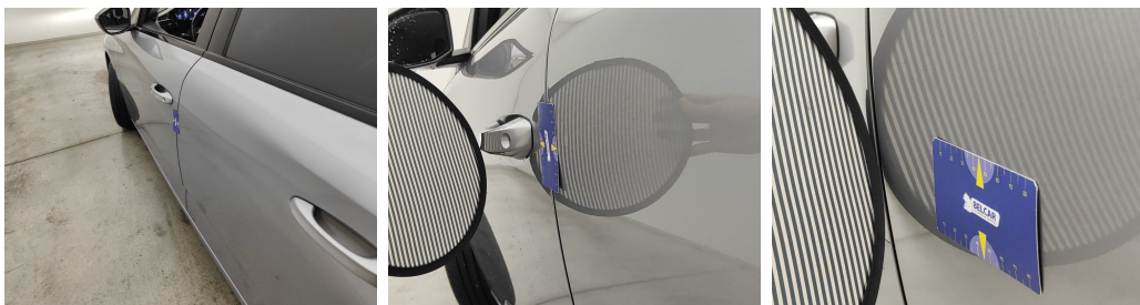
Door Rear Left // Painting-bad repair
