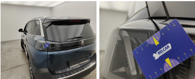
Light / Rear left / Replace-scratch
