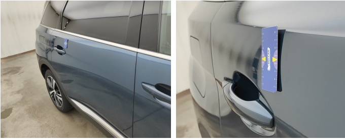
Door Rear Right // Painting-bad repair
