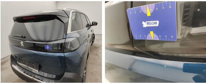
Light / Rear Right On Rear Bonnet / Replace-scratch
