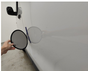
Wing Rear Left // Smart Repair Small-dent
