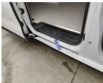
Rocker Panel Right // Smart Repair Medium-scratch + dent
