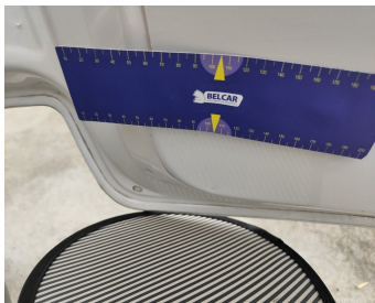
Rear Loading Door Right // Smart Repair Medium-scratch + dent
