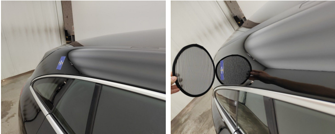
Roof // Smart Repair Medium-dent
