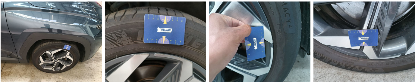
Wheel Two Tone Front Right // Repair-scratch
