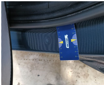
Rocker Panel Left // Smart Repair Medium-scratch + dent
